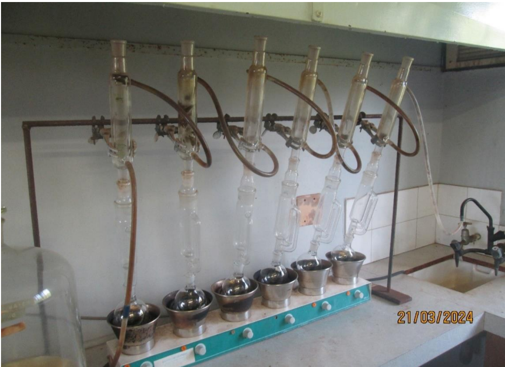
Figure 1. Extraction of Mycotoxins from Samples Using Soxhlet Extractor.
