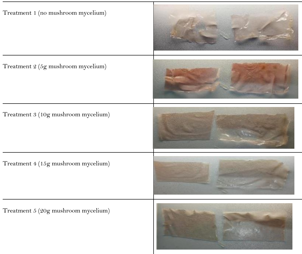
Figure 3. Durability of Oyster Mushroom mycelium bioplastic.
